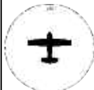
FIG. 5 An approved anti-collision strobe light system must project light 360° around the aircraft's vertical axis. One or more strobe lights can be used.
